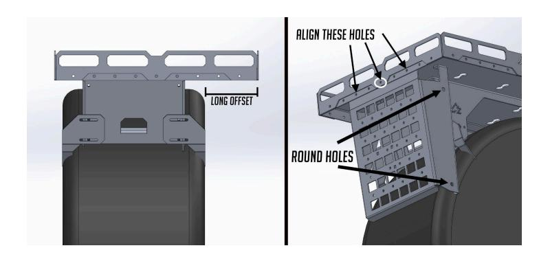
NOTE: It is very important to install into the correct holes before drilling the holes in the following step. Please see the large diagram below for a more detailed explanation. You will use the **third bolt hole** from the rear of the platform for the first bolt you install.
