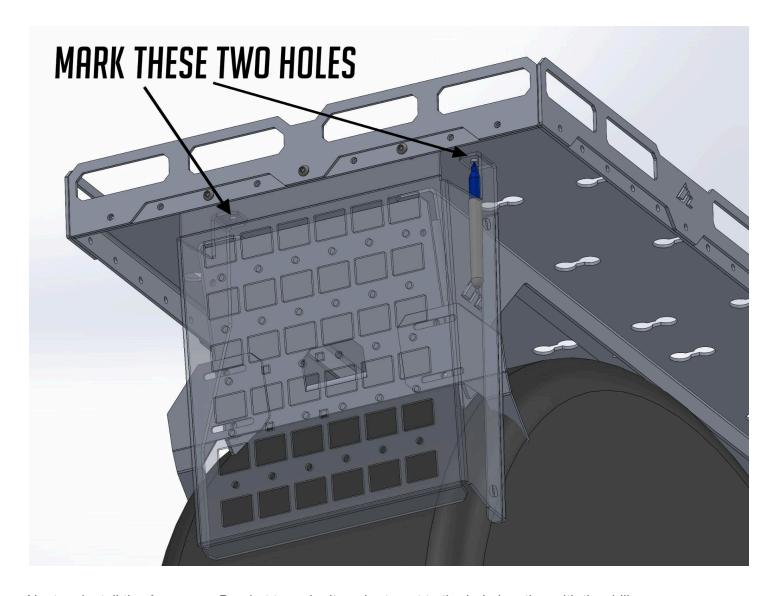
Next, uninstall the Accessory Bracket to make it easier to get to the hole location with the drill.
